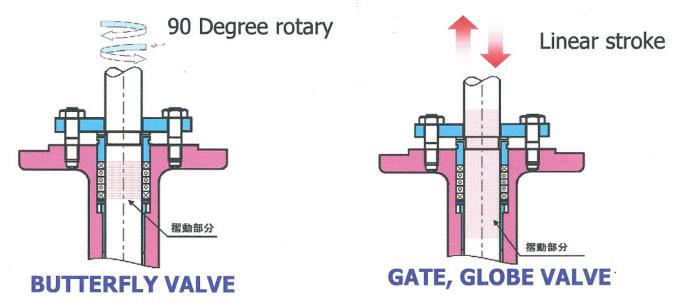
Rotary typed valve "Tritec" have been known for less load to gland packing and low emission comparing with gate and globe valve. It was proved from this test result.
